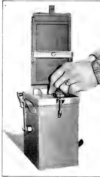
Introducing a plate into the tank. The handle is pulled back just long enough for the plate to pass through
